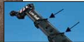
A-max extends only the inner-mid section of the boom for substantially increased capacities for in-close, maximum capacity lifts.
