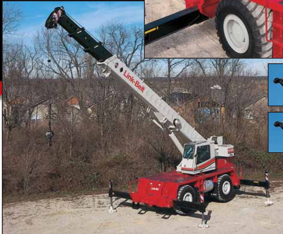
A-max extends only the inner-mid section of the boom for substantially increased capacities for in-close, maximum capacity lifts.
