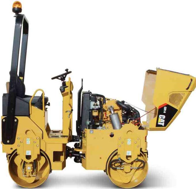
**Engine Enclosure.** Fiberglass engine enclosure pivots upward and locks open with a prop rod.
