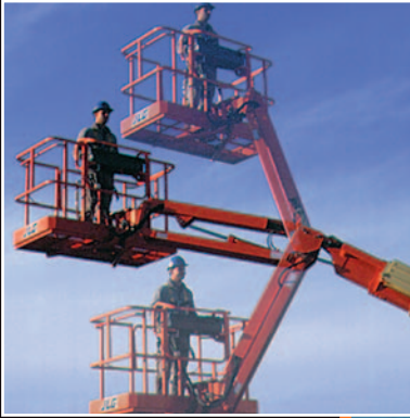
Articulating Jib Provides Reach Versatility
